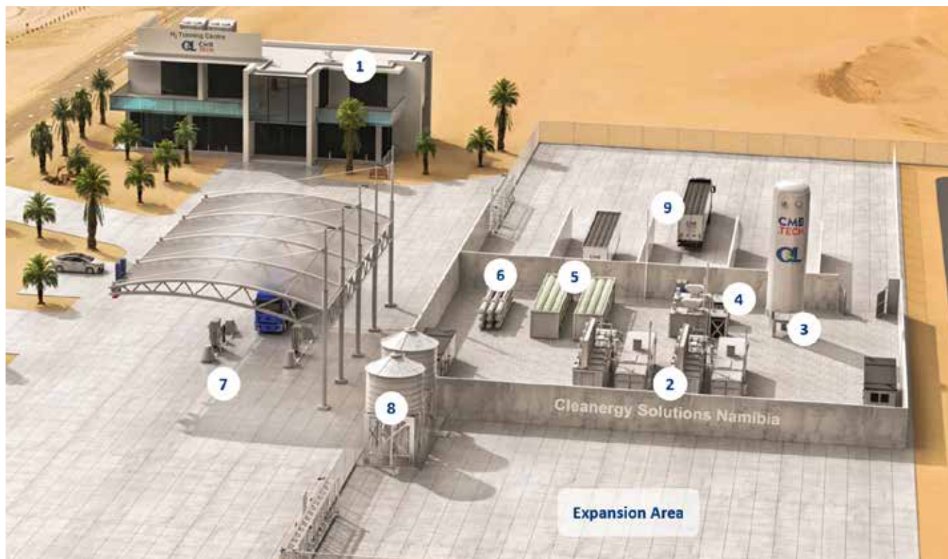
DEMO HUB ... The Cleanergy demonstration hub at Walvis Bay. 1) H2 training centre 2) H2 process and power containers 3) Low pressure buffer 4) Compressor 5) 300 bar buffer 6) 500 bar storage tanks 7) 350 bar dispensers 8) Water tanks 9) Tube trailers base
