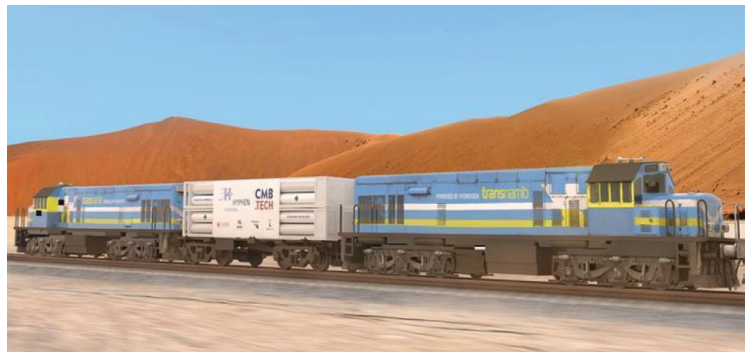
Visualisation of the HyRail dual-fuel hydrogen-diesel locomotive.
